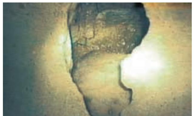
**Hole in pipe at joint**
